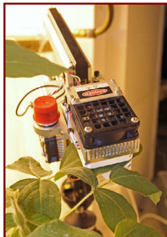
Fig. 3: Measurement of net carbon exchange rate using the LI-6400 system, mounted with a red/blue LED light source (set at 1500 \mu\text{mol s}^{-1} \text{m}^{-2} ).
