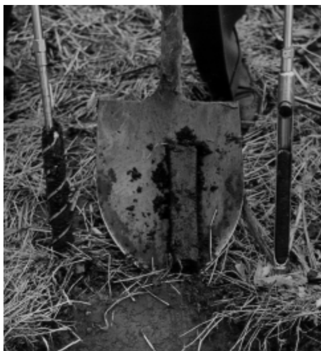
Figure 1. A soil probe, auger, or spade and knife should be used in sampling soils. The spade sample must be trimmed as shown.
