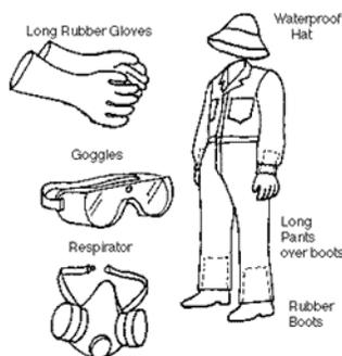
The pesticide label provides handling precautions, minimal **personal protective equipment (PPE)**, and other safety measures to minimize your exposure while handling pesticides. PPE comprises the clothing and devices you wear to protect your body from contact with pesticides. Wearing PPE can reduce exposure and lower the chances of pesticide injury, illness, or poisoning. **Basic protective work clothing consists of: a long-sleeved shirt, long pants, closed toed shoes, and socks.**
