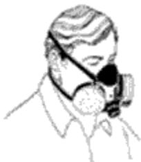
When you use pesticides, you may be exposed to toxic gases, vapors, particulates (solids or liquids), or all of these. A **respirator** is a safety device that protects you from inhaling contaminated air. The pesticide label states whether you must use a respirator and if so, which type. The respirator type is based on the pesticide formulation, application method, and environment where the application is made.
