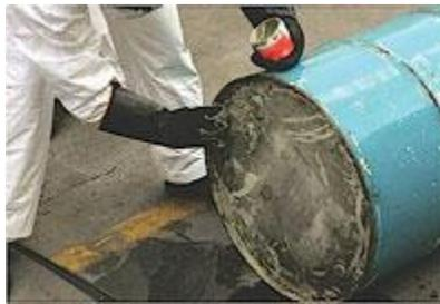
Plug a puncture to stop the spill
