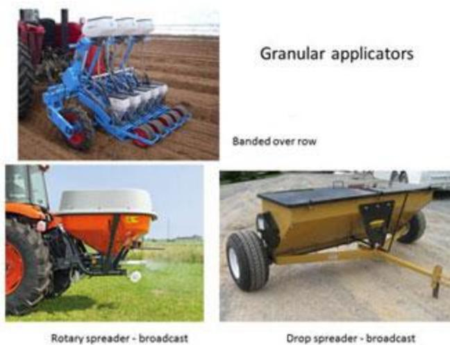
**Granular applicators** are available for either band or broadcast applications. They may be operated as separate units but often are attached to other equipment, such as planters or cultivating equipment, to combine two or more operations. Granular applicators usually operate by gravity feed and have an adjustable opening to regulate the flow.
