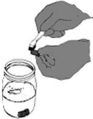
Nozzles are available in various materials: brass, aluminum, plastic, stainless steel, hardened stainless steel, and ceramic. Select the material best suited for the pesticide formulation being used.
