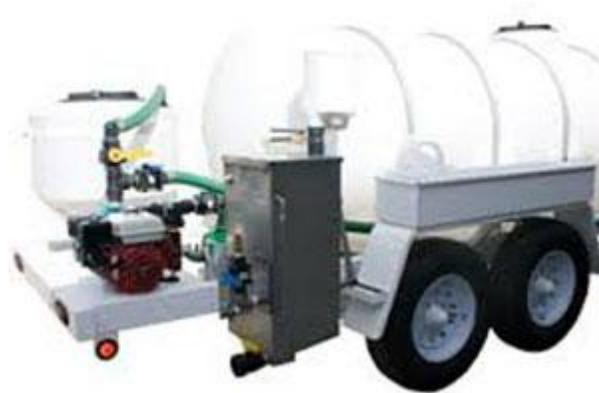
*Closed pesticide mixing system (PMB Supply)*
