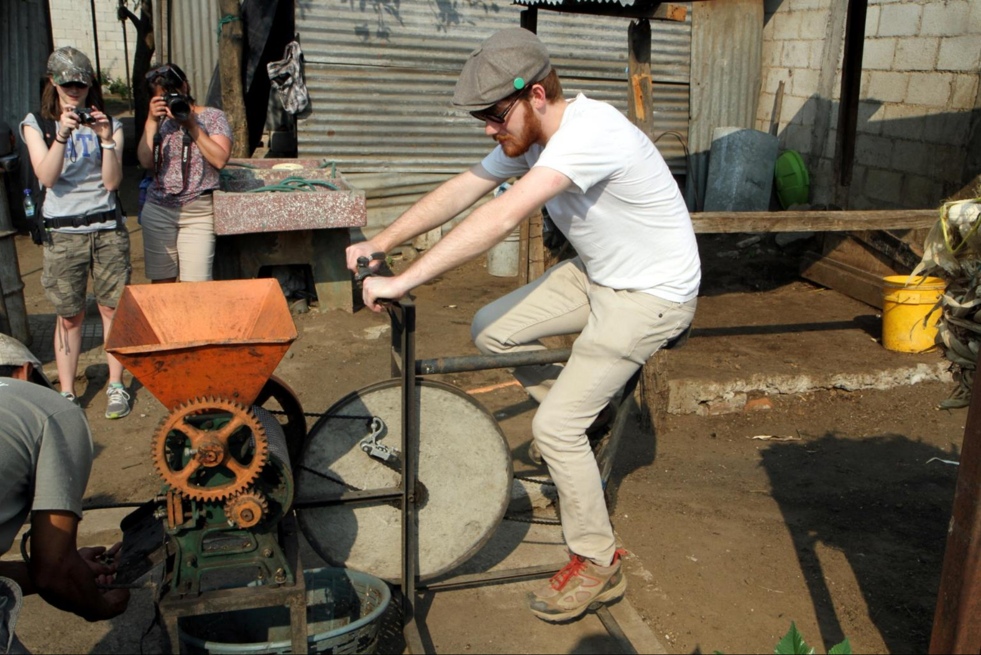
This grower employs a bicycle-like pedal powered fruit removal machine.
