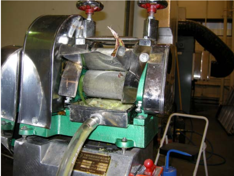
Figure 2. Single roll juicer used for experiments.
