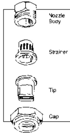
**Nozzle tips** break the liquid pesticide into droplets. They also distribute the spray in a predetermined pattern and are the principal element that controls the rate of application. Nozzle performance depends on: nozzle design or type, operating pressure, size of the opening, discharge angle, distance of nozzle from the target.
