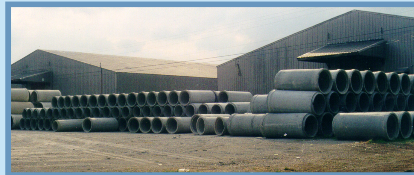
Storm-water drainage conduits are made of cast concrete.
