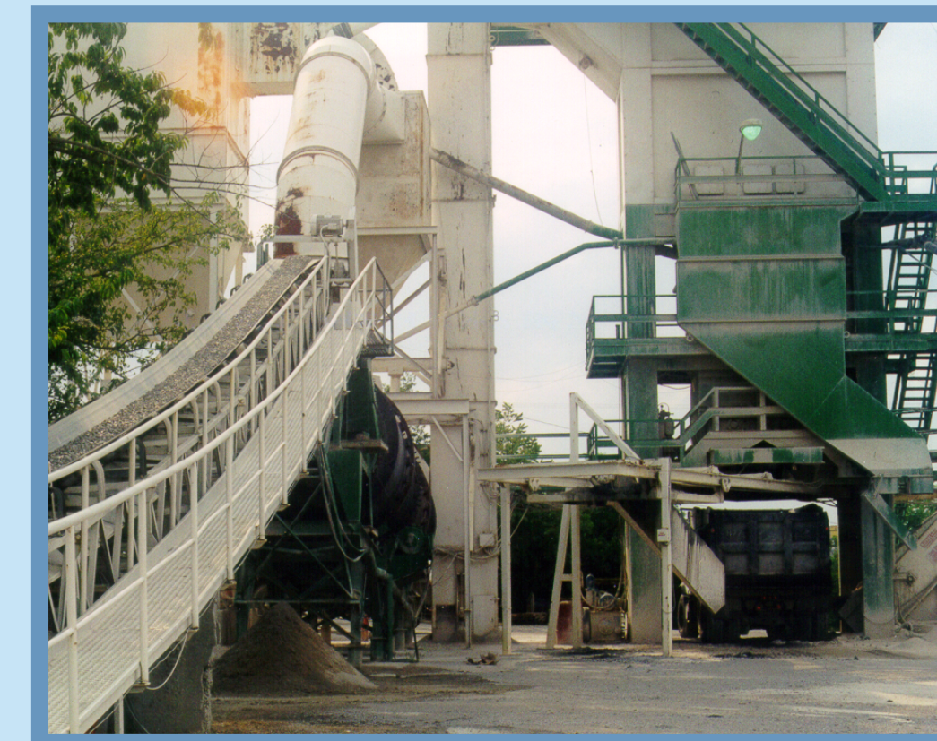
Crushed stone (on belt at left) is mixed (in black drum) with heated petroleum tar to make asphalt to be delivered in the truck (at right) for paving roads.
