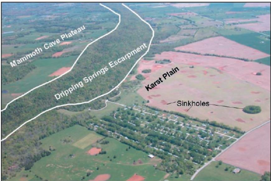
Figure 2. Oblique aerial view of karst plain, escarpment, and plateau areas. View toward east. Note ponding of water in sinks.
