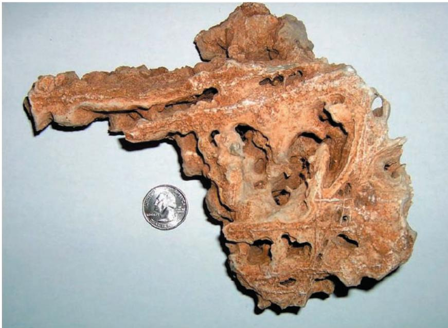
Figure 7. Hand sample of Ste. Genevieve Limestone showing complex dissolution in three dimensions.
