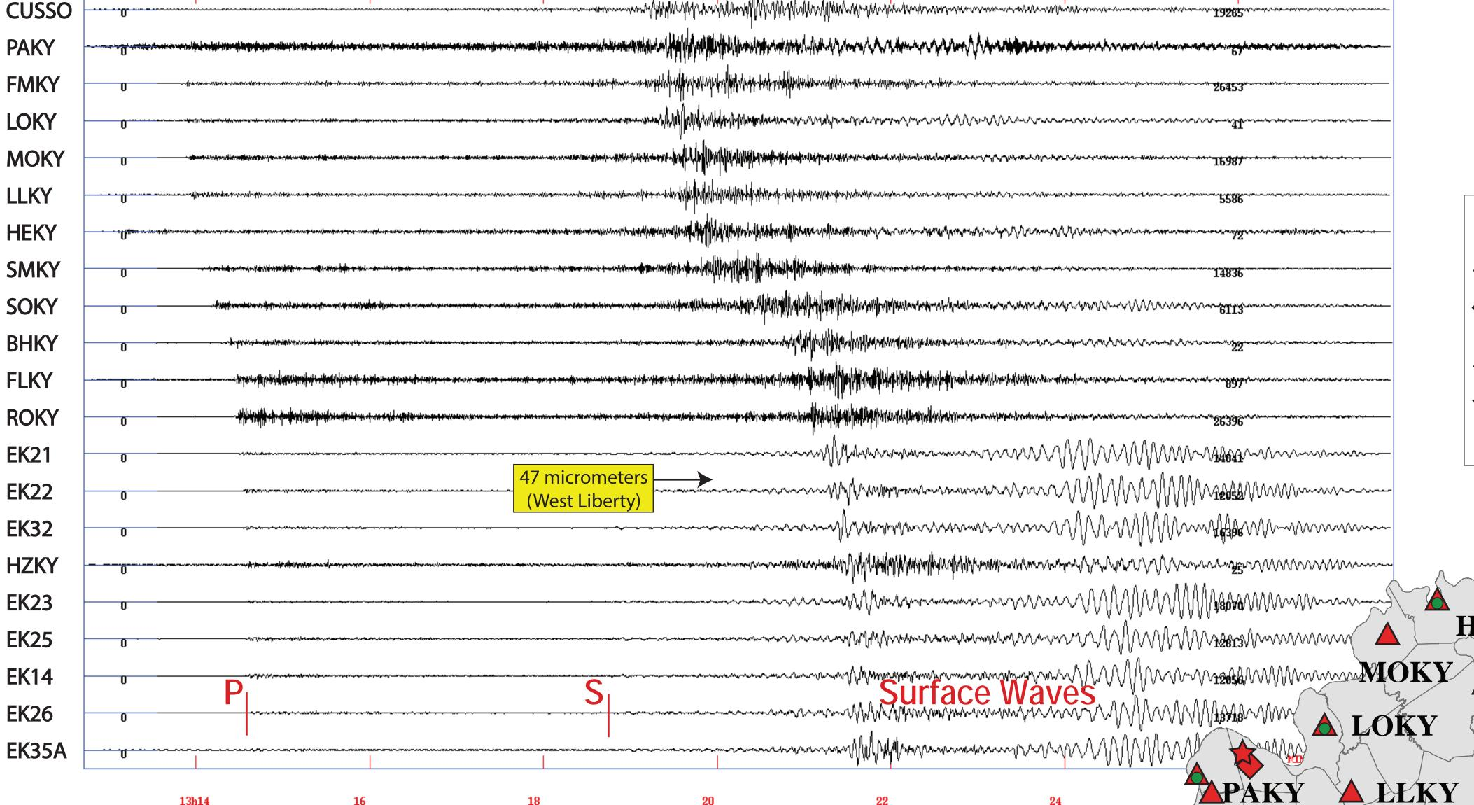
"P" and "S" mark P- and S-wave arrival times, respectively, at monitoring station EK26 in Louisa, Ky. Peak surface-wave displacement recorded at EK22 (West Liberty, Ky.) is labeled. Some differences in waveform appearances are due to the different types of instruments operated by the KSSMN.
