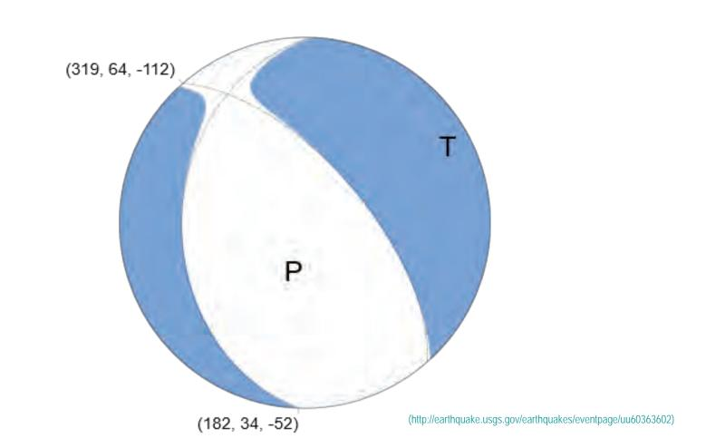
This focal mechanism, derived from seismograms, shows that predominantly normal-slip faulting occurred of a west- or east northeast-dipping fault plane.
