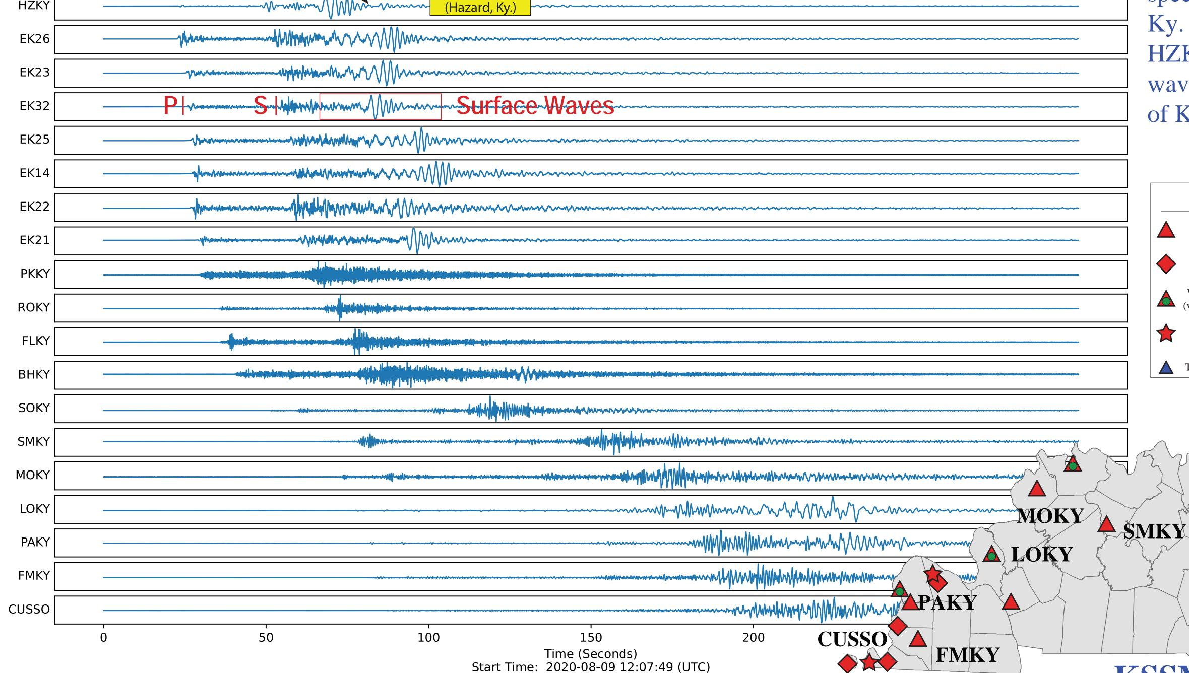
"P" and "S" mark P- and S-wave arrival times, respectively, at monitoring station EK32 in Jackson, Ky. Peak surface-wave displacement recorded at HZKY (Hazard, Ky.) is labeled. Some differences in waveform appearances are due to the different types of KSSMN instruments.
