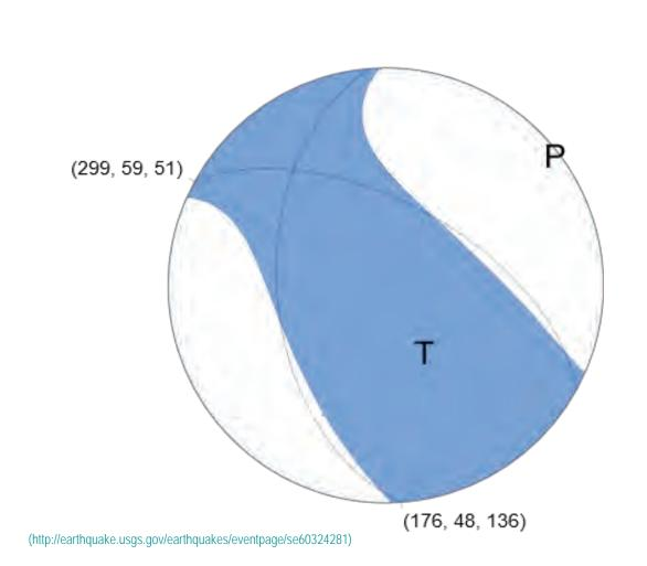
This focal mechanism, derived from seismograms, shows that oblique-reverse faulting occurred on a west- or northeast-dipping fault plane.
