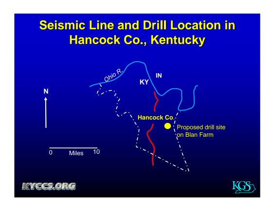
The proposed drill site ( yellow dot ) on the Blan Farm in eastern Hancock Co., Ky. The red line is the Gulf Oil and Production Co. Line 7 C, the nearest seismic data to the proposed site. The drill site lies approximately 4 miles to the east of the seismic line.
