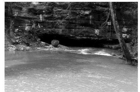
Nontoxic, colored dyes are added to springs to trace the flow paths of groundwater. Dark area in water is dye.
