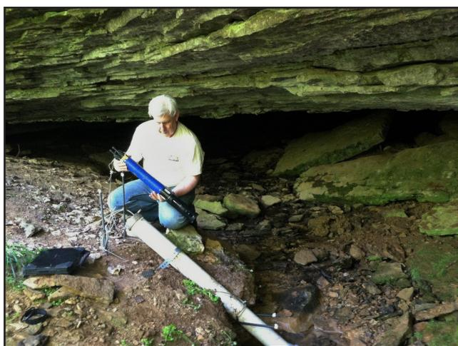
Figure 11. Kentucky Geological Survey hydrogeologist Chuck Taylor installs a multiparameter water-quality data sonde in water flowing out of a cave spring at The Homeplace on Green River.
