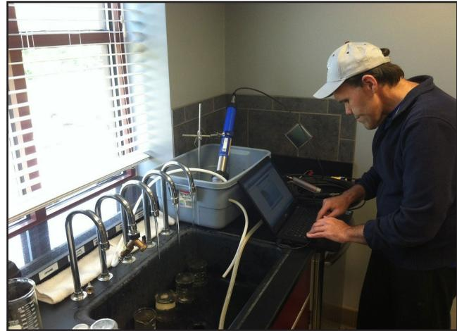
*Figure 9. Kentucky Geological Survey hydrogeologist Steve Webb calibrates a multiparameter water-quality data sonde to monitor changes in temperature, pH, specific conductance, and turbidity of water pumped from Head of Rough Spring to Hardin County Water District No. 1’s treatment plant near Cecilia.*
