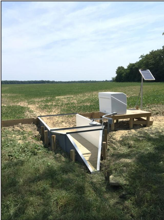
*Figure 17. One of six edge-of-field nutrient and sediment-loss monitoring stations in the lower Green River watershed.*
