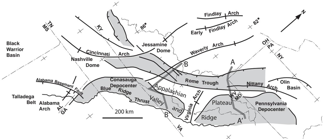
**Figure 2.** Structural base map of central and southern Appalachia Valley and Ridge, showing depocenters and Rome Trough (shaded) and arches (modified from Read, 1989a). Base map is not palinspastically restored. Location of schematic cross sections A-A' and B-B' shown.
