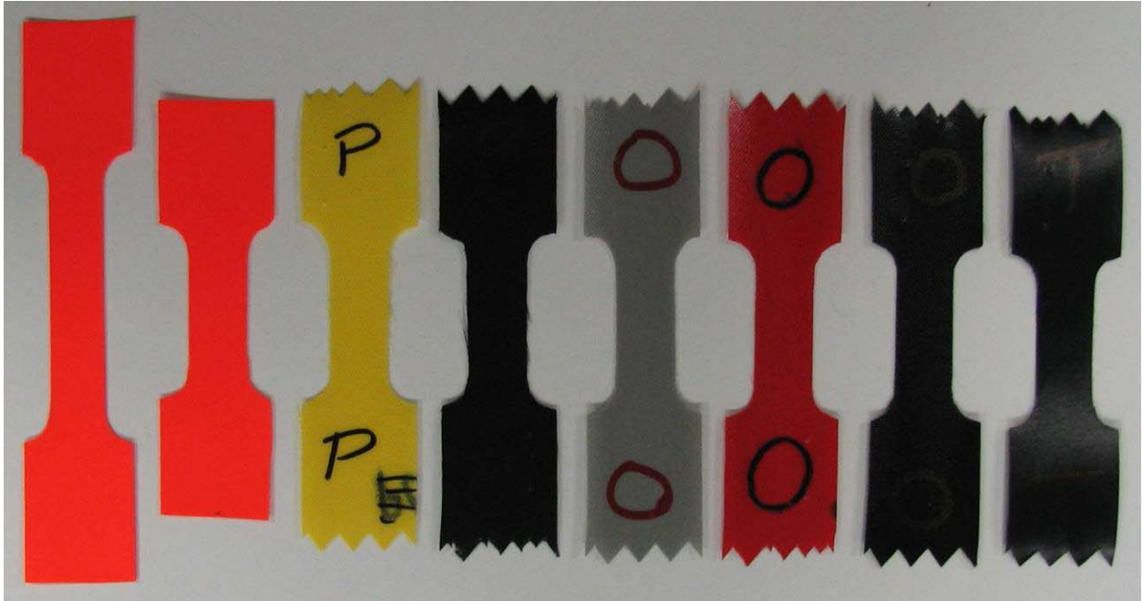
Figure 2. Tensile specimens before testing, in order from left: (Orange-L, Orange-S, Pack Cloth-Yellow, Pack Cloth-Black, Oxford-Grey, Oxford-Red, Oxford-Black, Tafetta-Black)
