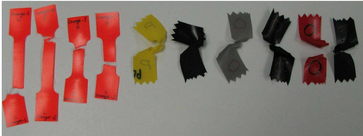
Figure 5. Tensile specimens after testing, in order from left: (Orange-L, Orange-S, Pack Cloth-Yellow, Pack Cloth-Black, Oxford-Grey, Oxford-Black, Oxford-Red, Tafetta-Black)
