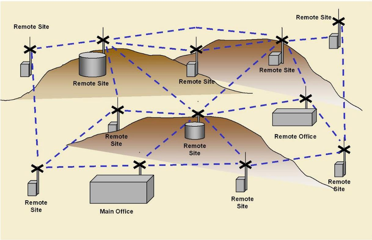
**Figure 2. Typical SCADA Communication Network Configuration**
