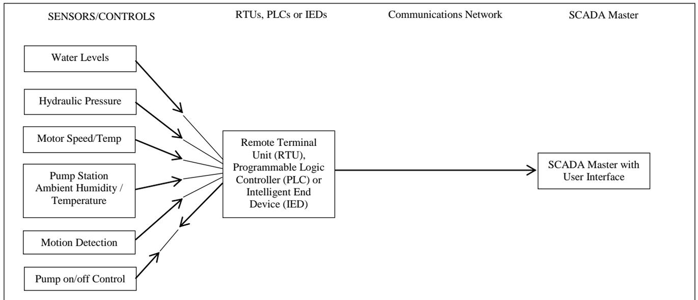
**Figure 1. SCADA Components**
