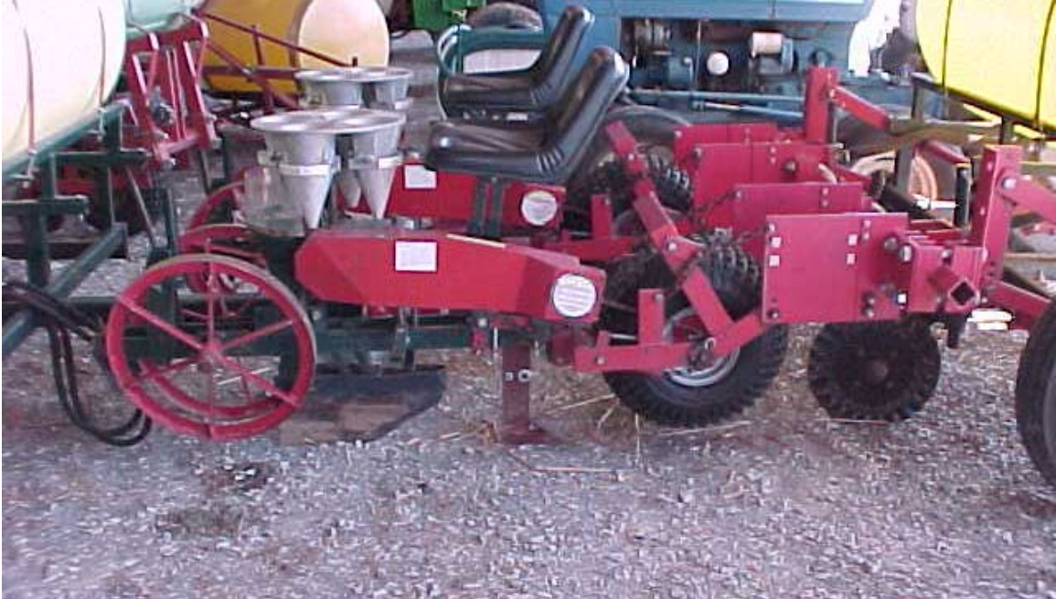
Figure 1. Two row Mechanical Model 6000 transplanter modified for use in no-till conditions.
