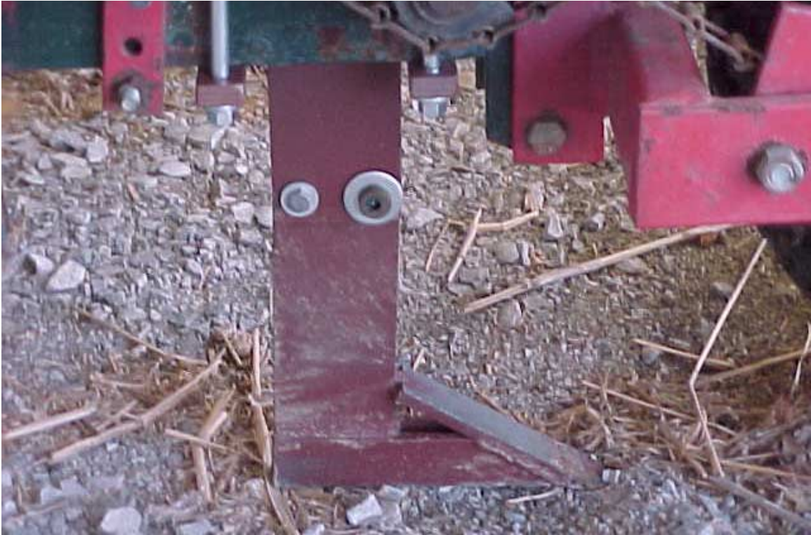
Figure 5. Subsurface tillage shank attached to unit frame.
