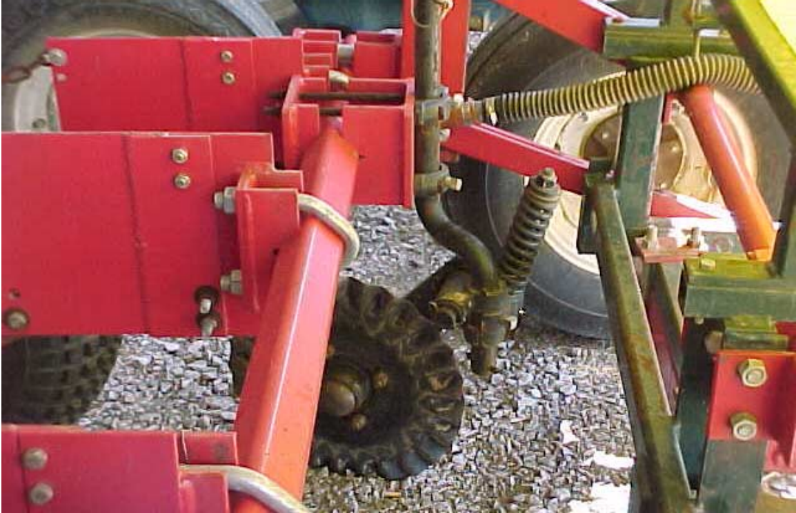
Figure 3. No-till coulters showing ripple blade
