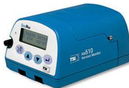
Aerosol TSI SidePak AM510 Personal Monitor
