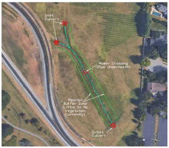
Figure 1b. Existing conditions at the stream consist of two inlet culverts, one outlet culvert (before the embankment located to the south), a mower crossing, and limited riparian vegetation.
