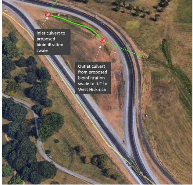
Figure 3. A portion of the flow passes under Alumni Drive (dashed green line at top of figure), enters a traffic island basin, and then passes under Alumni Drive again (second dashed green line from basin outlet) before entering the UT to West Hickman. The solid green line represents the proposed bioinfiltration swale.
