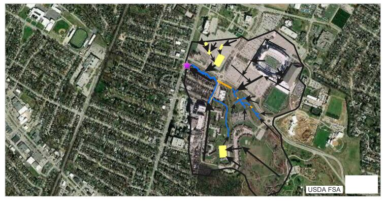
The goal of this map is to show the overall stormwater system that drains into Big Elm Fork. The arrows roughly represent the direction of stormwater runoff.
