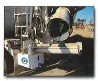
Figure 7. Chute washout box
