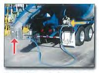
Figure 8. Chute washout bucket and pump
