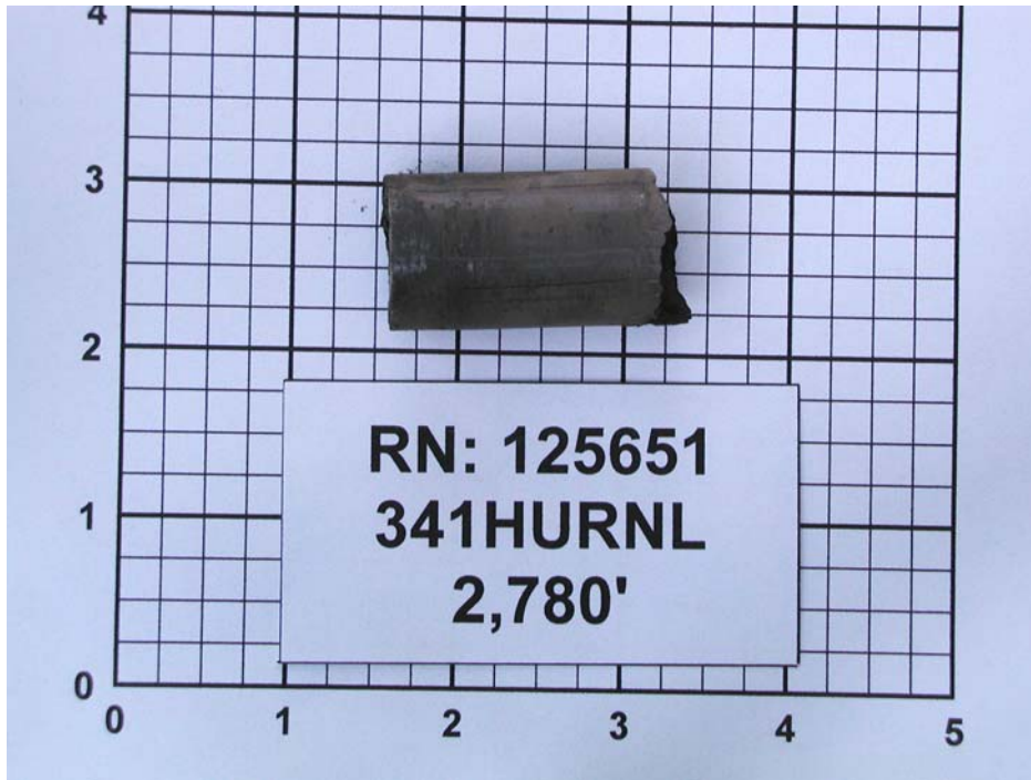
Sidewall core number 3 (0.25-inch grid).. This sample included a pyrite clast but is otherwise typical of the intact cores as submitted for analysis.
