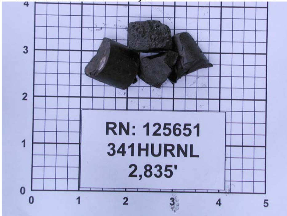
Sidewall core number 2 (0.25-inch grid). This sample exhibits an oily sheen characteristic of cores collected that were saturated with light hydrocarbons. This core is typical of the broken samples.
