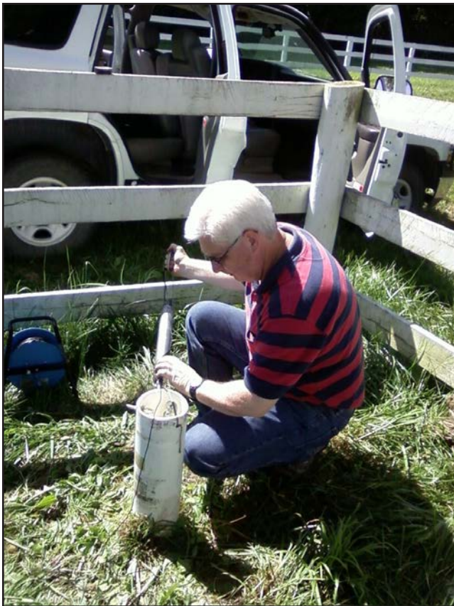
Figure 9. KGS hydrogeologist installs real-time monitoring equipment in a water well at the Kentucky Horse Park in Fayette County, as part of the Kentucky Groundwater Observation Network.
