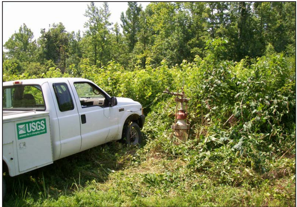
Figure 7. USGS personnel download data from a transducer installed in an abandoned gas well near West Point.
