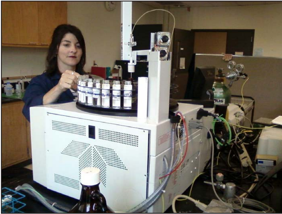
Figure 12. A KGS laboratory scientist runs groundwater samples from Muhlenberg County using the organic carbon analyzer.
