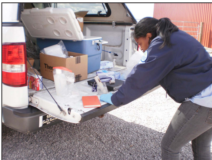
Figure 3. Groundwater Section personnel record pH, conductivity, and temperature at the Robey Farms monitoring network site in Logan County.
