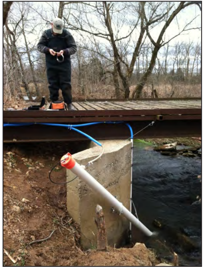
Figure 14. Water Resources Section hydrogeologist Steve Webb installs water-quality and water-level monitoring equipment at the Head of Rough Spring monitoring station in Hardin County.
