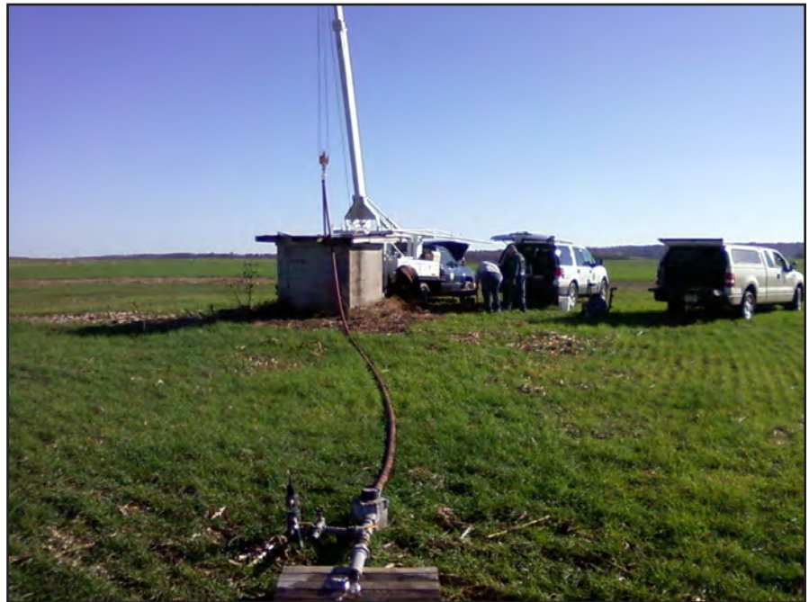
Figure 11. An aquifer test being conducted by KGS Water Resources Section scientists on an unused water well (located inside the concrete blockhouse) at the University of Kentucky Education and Research Center in Princeton.
