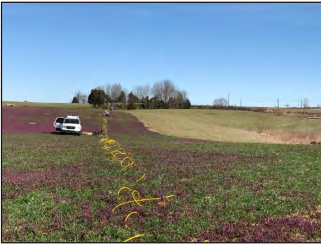
Figure 13. Hydrogeologists from KGS lay out electrodes and cables needed to conduct an electrical-resistivity survey to search for underground conduits containing groundwater at the farm at The Homeplace on Green River, near Campbellsville.
