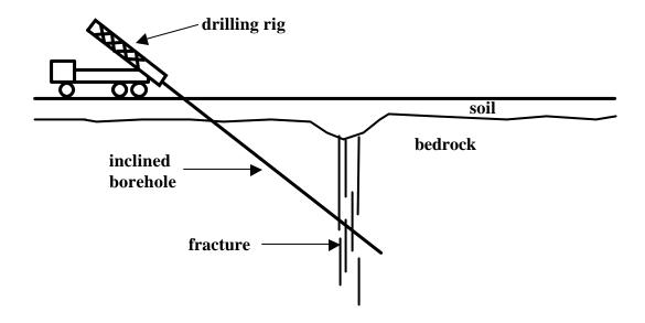
(B) Drill production well over the fracture discovered from the inclined borehole.
