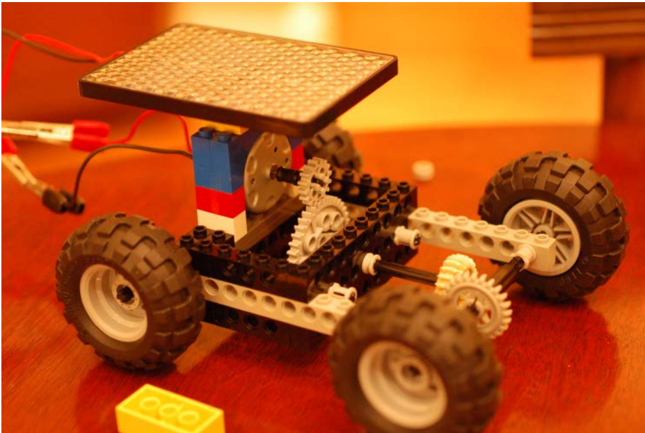
Figure 17. Working solar vehicle with small gear on motor and larger gear connected to gear assembly on front wheels axle
