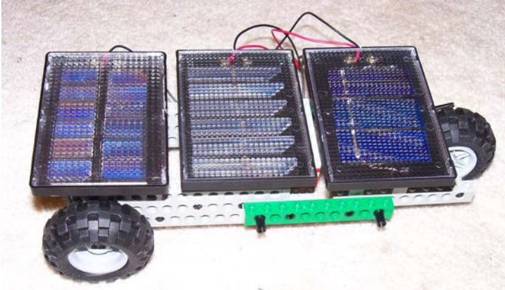
Figure 16. Sample solar vehicle with three wheels and three solar cells
