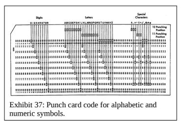
Punch card storage was not very dense by today's standards. The cards measured 3 <sup>1</sup>/<sub>4</sub> by 7 3/8 inches,<sup>22</sup> and a deck of 1,000 was about a foot long. Assuming that all 80 columns are fully utilized, that works out to about 48,000 characters per cubic foot, which sounds good until we compare it to PC thumb drives which currently hold up to 8 billion characters.
