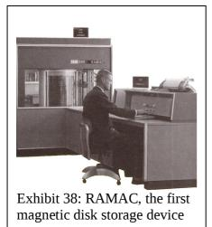
IBM shipped the RAMAC on September 13, 1956. The disk could store 5 million characters (7 bits each) using both sides of 50 two-foot-diameter disks. Monthly rental started at USD 2,875 (USD 3,200
