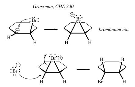
I've drawn the Br<sup>-</sup> ion attacking the left-hand C atom in the bromonium ion. It could equally well attack the right-hand C atom. The bromonium ion is achiral, and the product is chiral, so the product is obtained as a racemic mixture. One enantiomer is obtained from attacking one C of the bromonium ion, and the other is obtained from attacking the other C.
