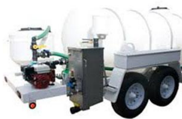
Closed pesticide mixing system (PMB Supply)
