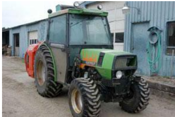
Spray tractor with enclosed cab (Univ. Vermont)
