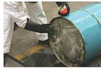
Plug a puncture to stop the spill
