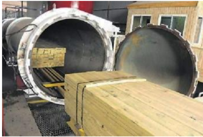
Lumber going into a pressurized treatment cylinder (image: jamaicaobserver.com)
