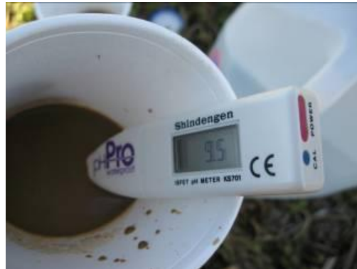
A handheld pH meter can help you quickly determine the soil pH, and thus, the risk of ammonia injury to germinating and seedling corn.
