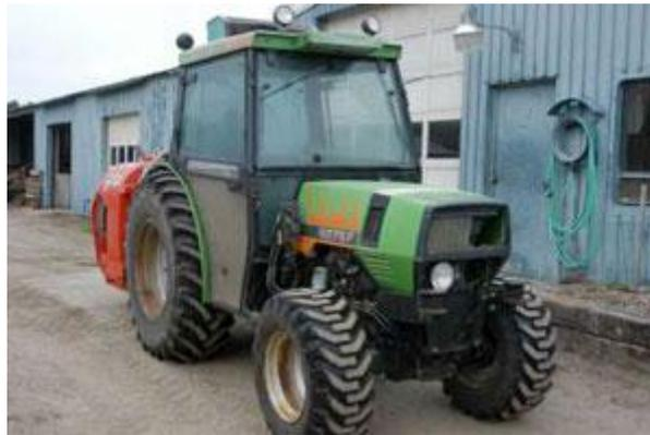
*Spray tractor with enclosed cab (Univ. Vermont)*
