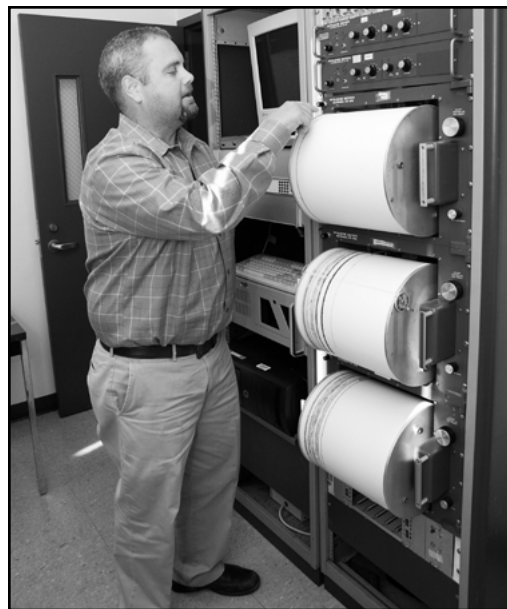
Jonathan McIntyre checked the operation of older seismic recording instruments in the Geologic Hazards Section.
