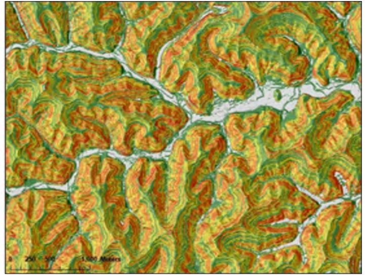
Figure 3. Example of mapped landslide deposits in northern Kentucky (left) and a landslide-susceptibility map of eastern Kentucky (right). The susceptibility map shows the probability that the slope factor of safety is less than 1. Reds and oranges are high probability and yellows and greens are lower probability. These types of maps are useful for land-use planners, engineers, geologists, emergency management officials, and others needing landslide hazards information.
