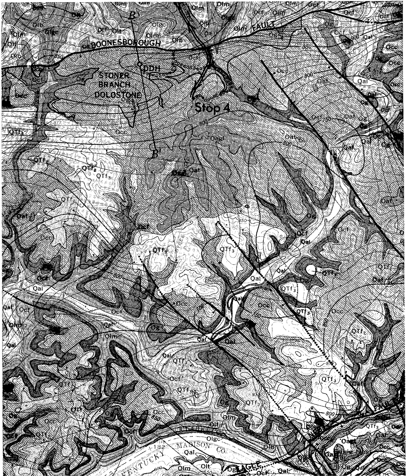
Figure 10. Geologic map of part of the Winchester quadrangle (modified from Black, 1974). Scale 1:24,000. Structure contours on top of the Garrard Siltstone south of the Boonesborough fault; on base of the Brannon Member of the Lexington Limestone to the north; contour interval 10 feet. Open circles near stop indicate route of walking traverse. DDH is location of U.S. Geological Survey Allen No. 1 diamond-drill hole. See Plate 2 for explanation of bedrock symbols and lithological descriptions; cross section B-B' is shown on Figure 3.
