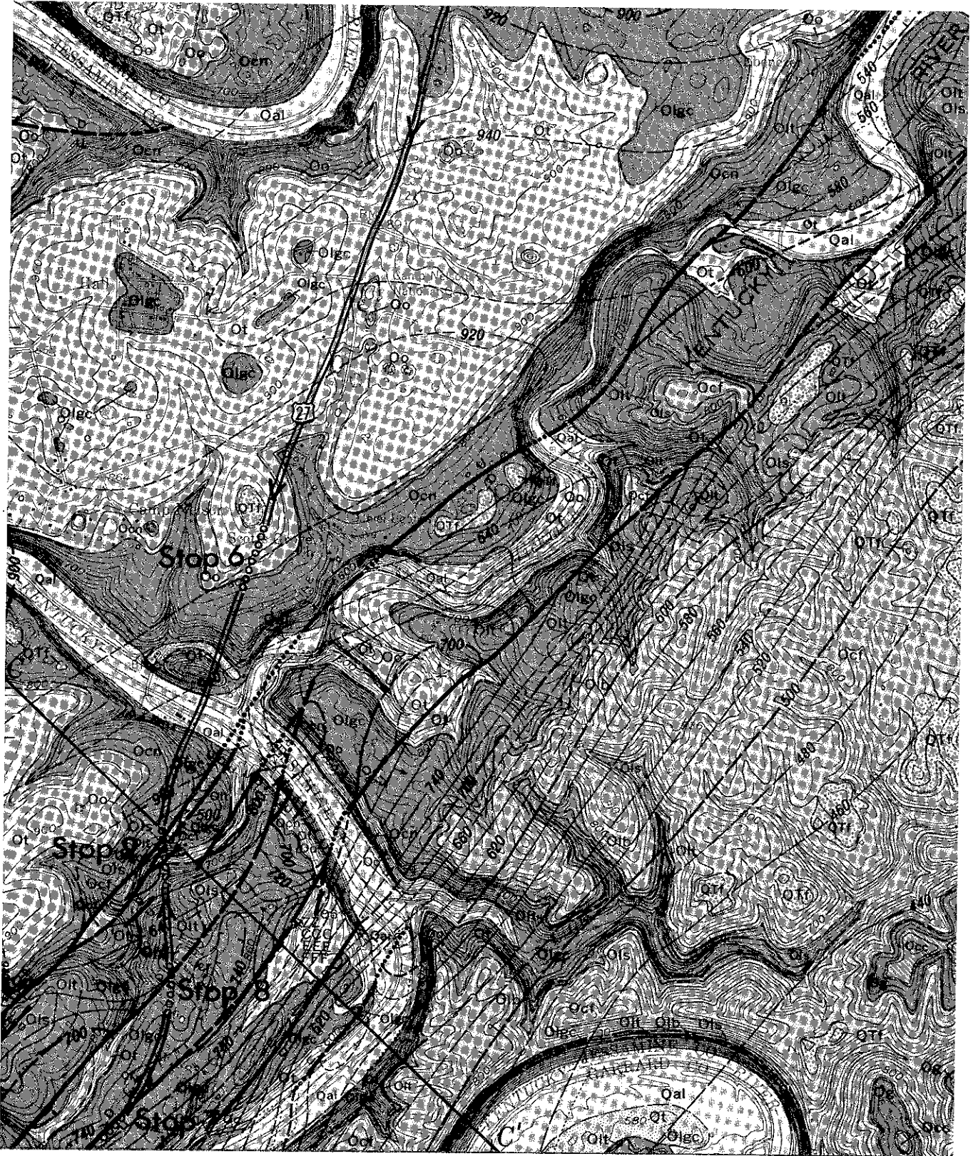
Figure 13. Geologic map of part of the Little Hickman quadrangle (modified from Wolcott, 1969). Scale 1:24,000. Structure contours on top of the Tyrone Limestone; contour interval 20 feet. Open circles near stops indicate route of walking traverses. See Plate 2 for explanation of bedrock symbols and lithologic descriptions; cross section C-C' is shown on Figure 3.
