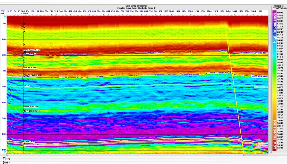
The Upper Knox has lower relative impedance than the Lower Knox. The results do not suggest lower impedance surrounding the fault location.
