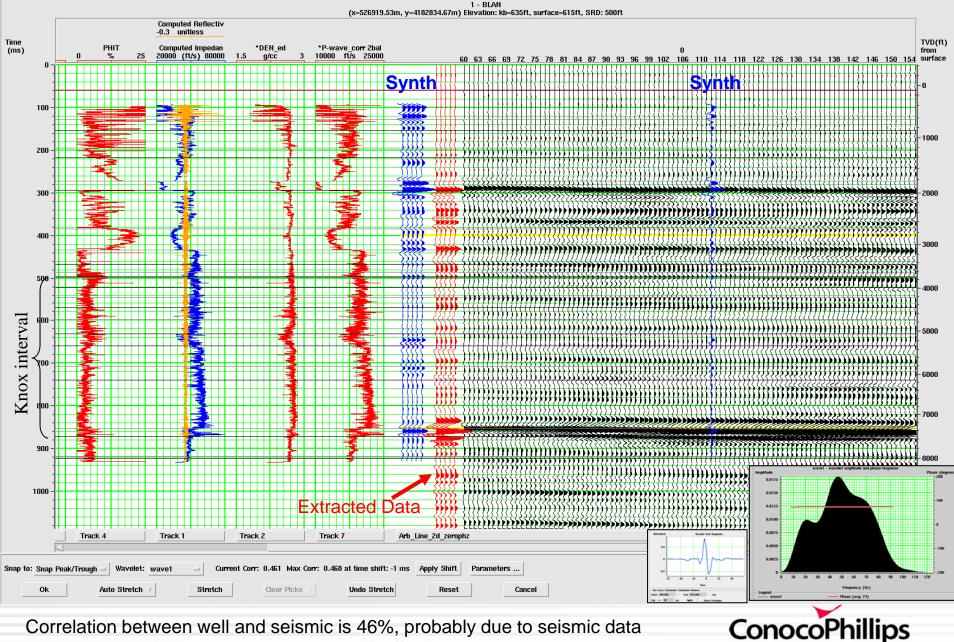
Correlation between well and seismic is 46%, probably due to seismic data quality and the fact that the well is ~1200 ft off the seismic line.
