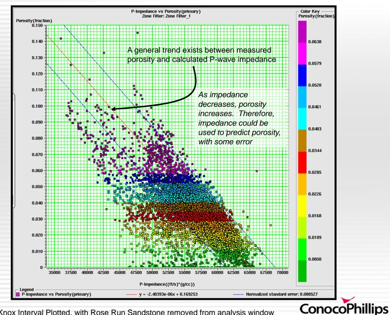
Knox Interval Plotted, with Rose Run Sandstone removed from analysis window
