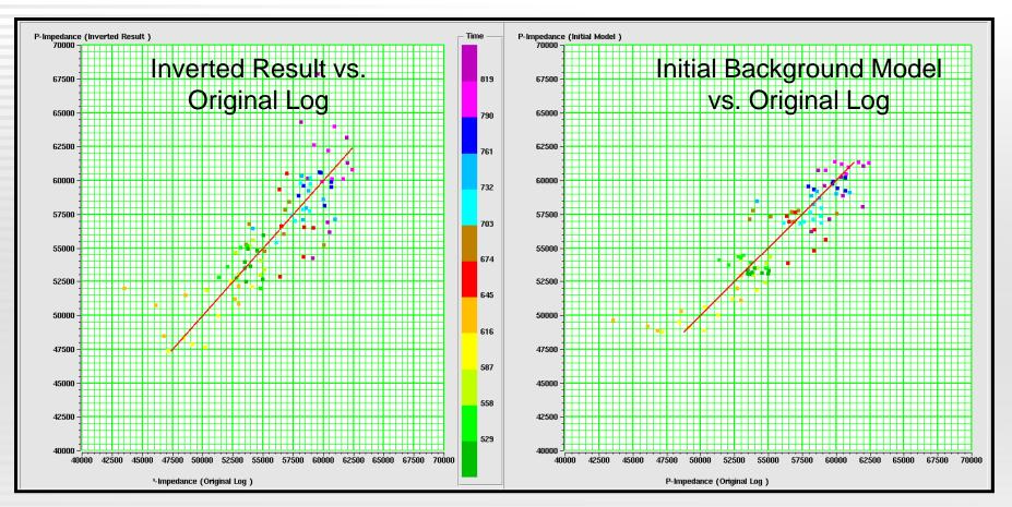
The inverted results for the Knox formation (both upper and lower) show about the same amount of error, but results are more scattered than the plot of the initial background model vs. original log. This indicates that the seismic is not adding any additional accuracy to our inversion.
