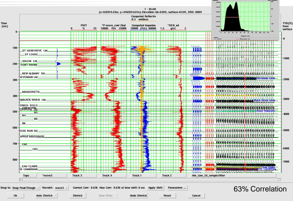
Seismic data filtered 0-12.5-38-55
