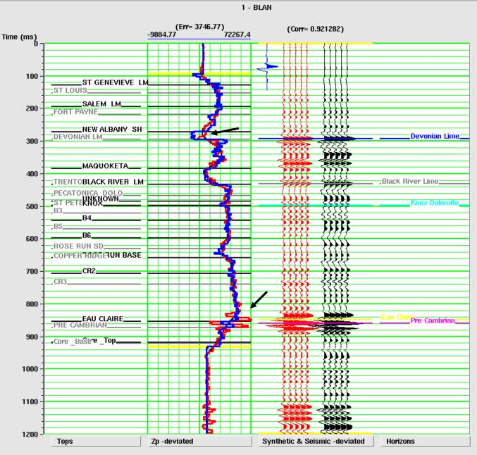
Bandlimited Inversion with 35Hz High –Cut Frequency Constraint.
