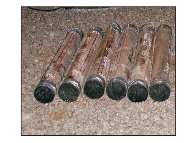
A 30 ft core of the New Albany Shale was cut in the Marvin Blan #1 well to evaluate its capacity as both a CO<sub>2</sub> storage reservoir and reservoir seal. This research is being conducted by KGS separately as a study of CO<sub>2</sub> storage and enhanced gas recovery from organic-rich Devonian black shales in Kentucky.
