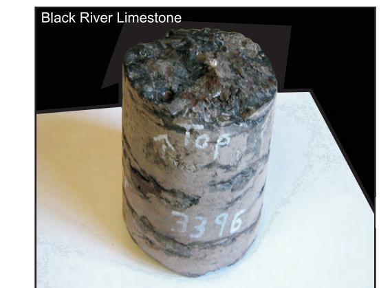
A 60 ft core of the Black River Limestone was cut in the Marvin Blan #1 for analysis as a reservoir seal. A correlative core form the #1 WAD showed half of the samples with vertical permeability less than 0.10 md with associated porosity averaging 4.6%.
