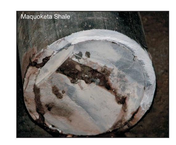
A 30 ft core of the Maquoketa Shale was cut in the Marvin Blan #1 well to evaluate its capacity as a CO<sub>2</sub> storage reservoir seal.
