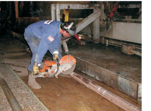
Core recovered in aluminum sleeve was cut into 3-foot sections for shipping
