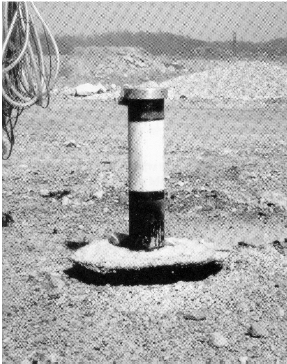
Figure 8. Settlement of the mine-spoil surface, as indicated by the movement of the cement surface seals.
