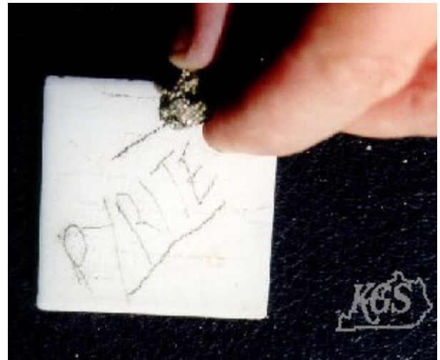
Pyrite has a brown to black streak (white unglazed tile is a streak plate).
