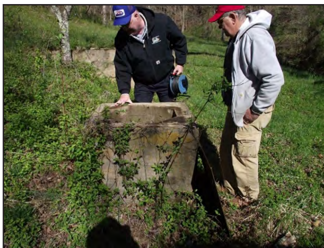
Figure 7. Bart Davidson and well owner Walter Black check the water level in a hand-dug well in Boyd County near Ashland.
