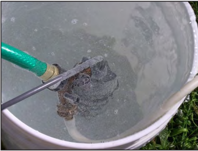
Figure 9. Effervescence from methane in purge water from a domestic drilled well in Johnson County.
