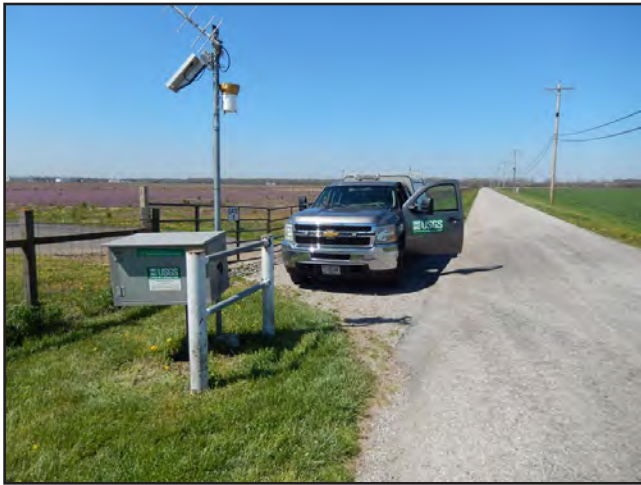
Figure 6. A USGS station measures and transmits groundwater levels in real time.
