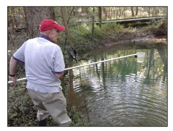
Figure 13. Kentucky Geological Survey geologist Richard Smath assists with sampling the McConnell Spring bluehole in Lexington using a telescoping sampling beaker. The instrument on the tree in front of him records basic field parameters of the water, including temperature, conductivity, and pH. Flow of the spring is also estimated before the sample is taken.
