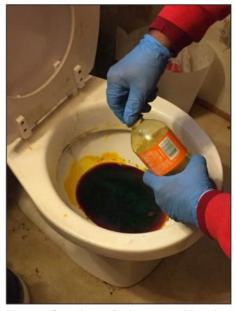
*Figure 5. Groundwater Section personnel introduce tracer dye into a toilet to check for leaks in a septic system during the Craft Lane investigation.*
