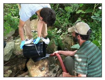
Figure 12. Kentucky Geological Survey karst hydrogeologist Ben Tobin and geologic technician Adam Nolte prepare to flush a fluorescent tracer dye into the partly blocked swallet (throat) of a sinkhole at The Homeplace on Green River.
