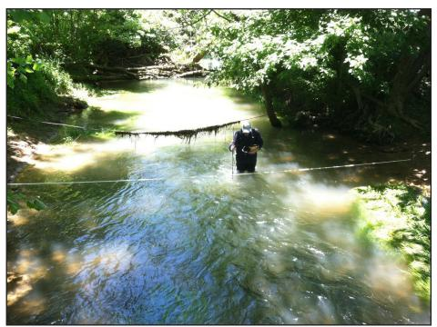
*Figure 10. Kentucky Geological Survey hydrogeologist Steve Webb measures discharge in the outlet channel of Head-of-Rough Spring near Cecilia.*
