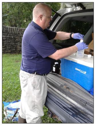
Figure 14. Kentucky Geological Survey geologist Bart Davidson adds nitric acid to a sample from Russell Cave Spring in Lexington. The acid reduces the pH of the sample to prevent bacteria from growing in the water before it is analyzed for total metals by the Environmental Services Branch laboratory in Frankfort.
