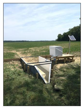
*Figure 17. One of six edge-of-field nutrient and sediment-loss monitoring stations in the lower Green River watershed.*
