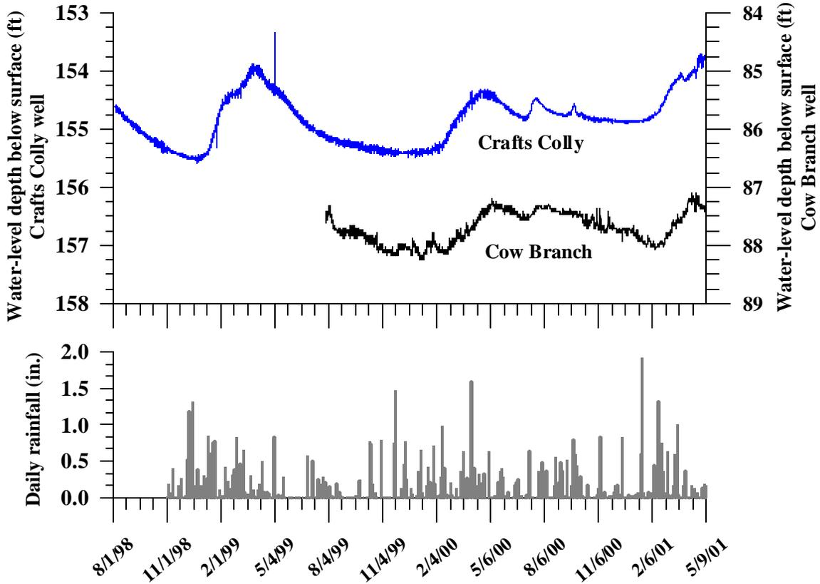
Water levels in Letcher County monitoring wells. The two graphs above are compiled from data collected from two wells penetrating abandoned mines in the Elkhorn No. 3 coal seam. The two wells are separated by a distance of approximately 2.5 miles.
