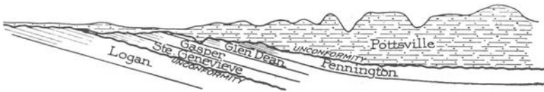
Fig. 7. Diagrammatic section across the eastern Kentucky coal field from South Portsmouth south eastward. Shows the unconformable relation of the Mississippian and Pottsville (coal measures).
