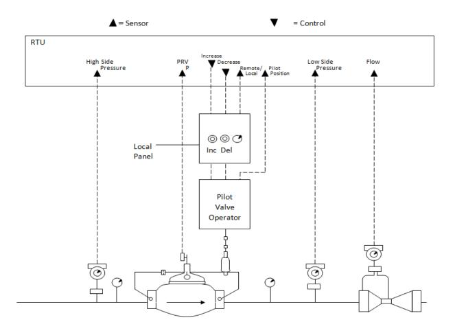
Figure 2. Typical PRV controls and instrumentation
