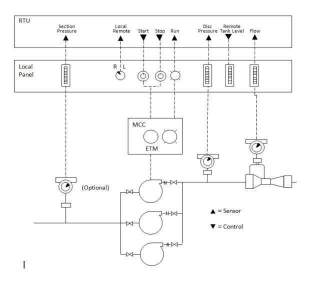
Figure 1. Typical pump station controls and instrumentation
