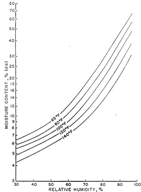
Fig. 3. Equilibrium moisture content as a function of temperature and relative humidity from combined data of Jeffrey (1940) and Locklair, et. al. (1957).
