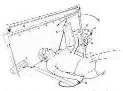
Figure 2 Illustration of proprioception testing device. a, Rotational transducer [1:3 mechanical speed-reduction gear-train]; b, motor; c, moving arm; d, control panel; e, digital microprocessor; f, pneumatic compression device; g, handheld disengage switch; h, pneumatic compression sleeve. Threshold to detection of passive motion is assessed by measuring angular displacement until subject senses shoulder motion.
